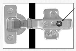
Turn screw indicated to adjust door in/out.
