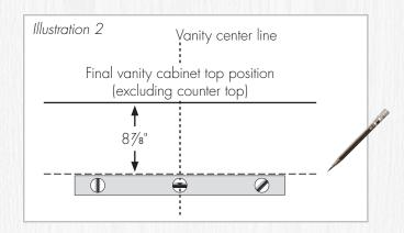
mark the wall for drilling into wall studs. Drill 3/16" pilot holes into wall and wall studs for 5/16" lag screws. **It is important to drill into stud center.** If installing an ensemble consisting of multiple components, carefully plan mounting bar placement for all cabinets first.
