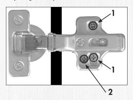
Loosen screws (1) on both hinges. Turn screw (2) equally on each hinge to move both hinges up/down.
