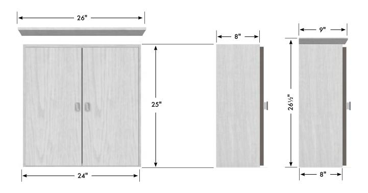
2 adjustable position shelves; 3/8" thick frosted acrylic, radiused front edge.
